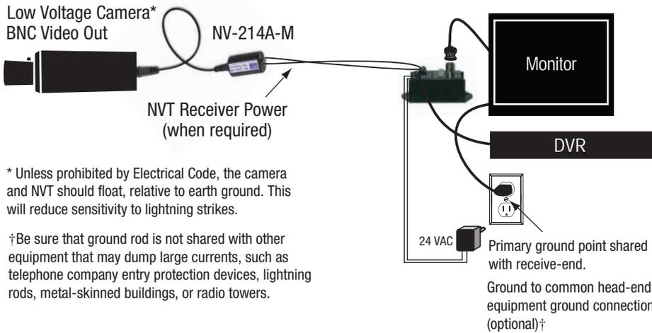
\* Unless prohibited by Electrical Code, the camera and NVT should float, relative to earth ground. This will reduce sensitivity to lightning strikes.
